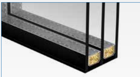
3-glass packet 4/14/4/14/4 INCREASED THERMAL INSULATION
